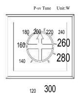
Note: To protect the motor, set the arrow number as the same as the motor nominated power. Whenever overload occurs the drive will turn out to be the protection mode.
