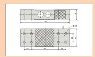
Dimension (mm): Size: 125x40x24(mm) Thread hole: M6
